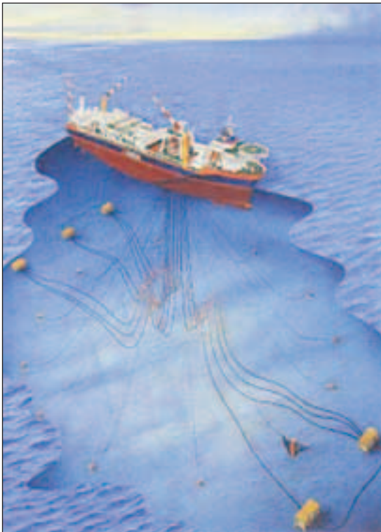
Figure 17. Example of a floating production facility.
